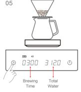
After brew is finished, short press to stop timing. Weighing panel shows your brewing data precisely.
