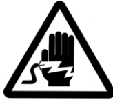
Caution: Electrical Shock Hazard!
