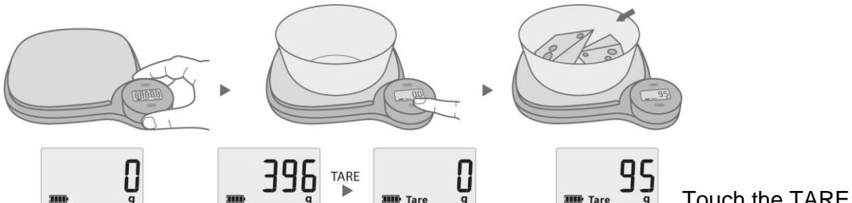
Touch the TARE button and the display shows zero "0" and clears the weight of container.
