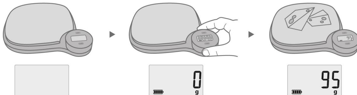
Place the scale on a hard & flat surface. Turn the knob clockwise until you see zero in the display.
