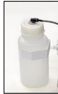
Fig. 6: Condensate collection vessel
