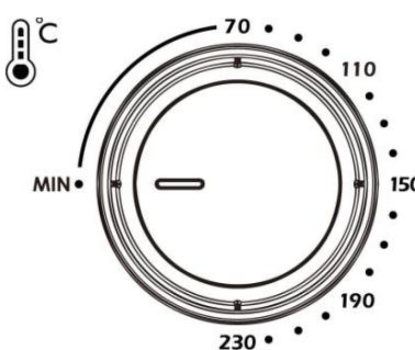
To adjust the temperature, not for switching off of the device.
