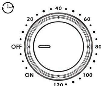
Set the desired time clockwise, the control lamp lights up.
