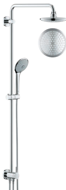
27 421 001 Euphoria 180 Shower system with diverter hand shower Euphoria 110 Massage 450 mm shower arm with 9.5 l/min GROHE EcoJoy
