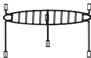
Grill Rack( Only be used in grill/convection function and be placed on the glass tray )
