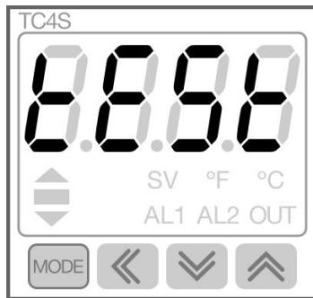
If you see **TEST** on the screen while working with the bowl, this means that the controller is now in test mode.
