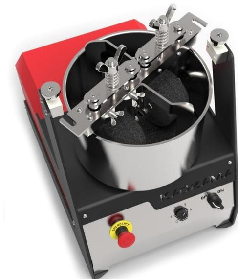
7.3. Before starting the rotation, you need to turn on the circuit breaker located on the rear wall of the body (under the casing). Also check button (4): if it turned on — rotate it clockwise to turn off.
