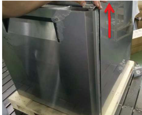
2) Remove the top hinge from the unit.
