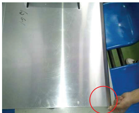
6) Take apart the door bushing from the bottom right hand side of the door.
