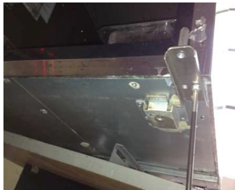
4) Unscrew the screws located on the bottom right hand hinge.
