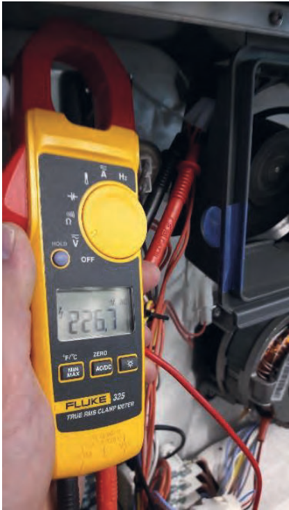
Test 1 Back cooling 230 V AC power supply
