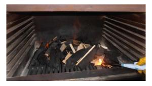
After the ignition door should be closed and coal should be waited to become incandescent. Approximately 30-40 minutes after, the coal become incandescent. Coal should be spread well with the help of coal tongs.
