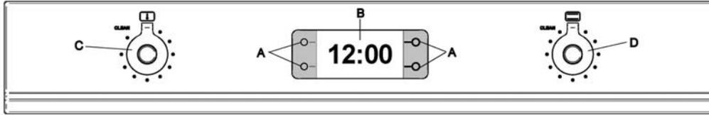
**A** Touch control areas    **B** LCD Display    **C** Temperature knob    **D** Cooking modes knob
