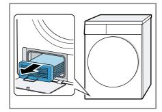
4. Clean the heat exchanger from all sides under running water and dry
