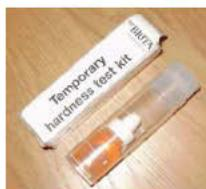
Measure the system water hardness in German degrees - °dH (taking it from a tap) using the supplied kit following the enclosed instructions.
