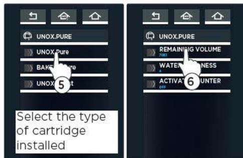
Select the type of cartridge installed
